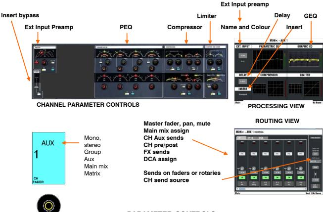
**PARAMETER CONTROLS** - Press a **GP**, **AUX**, **FX**, **MAIN** or **MTX** (Mix) master **SEL** key to access the parameters for that master using the analogue style controls in the processing block to the left of the screen. Every mix master has both a PEQ and a third octave GEQ as well as compressor, limiter, delay, external input and insert capability.
